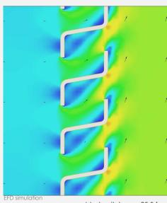
blade pitch 25.5 [mm] blade depth 25 [mm] min. built-in depth 50 [mm]
